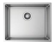
AISI 316 L Material Finishing Brushed Inner corners R 10 mm welded Overall dimensions 540 x 440 mm 500 x 400 mm Basin dimensions 200 mm Bowl depth Standard Strainer 3 ½" Cabinet size 600 mm Cod. **BI 5040 MR** Top mount Flush mount Cod. **BG 5040 MR**
